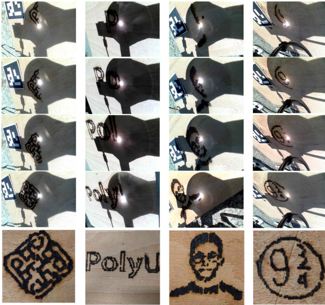
Fig. 14. Results of the solar painting experiments. The robot path is planned according to the feature points extracted from the target pattern.
